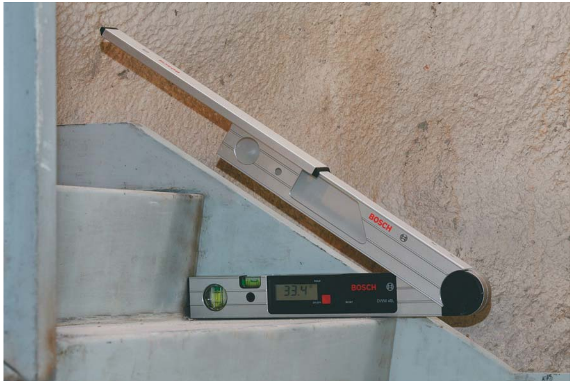
Above: Digital level angle finder. Below: Digital metal detector capable of locating metal reinforcement in concrete.
